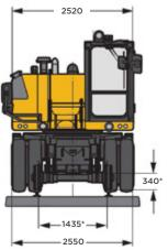
\*without outriggers / Symetric Rail mm
